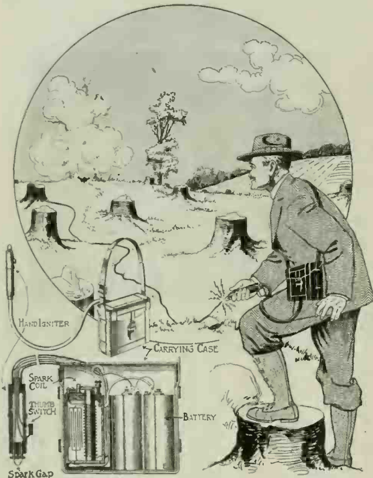
A New Electric Fuse Igniter for Blasting. It Produces a Shower of Sparks Between the Ignition Electrodes Whenever the Button Is Depressed. The Batteries and Spark Coil Are Carried in a Small Case Slung Over the Shoulder
