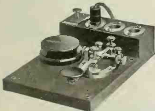
A Code Teaching Instrument Provided With Plug Switch for Battery and Omnigraph.
