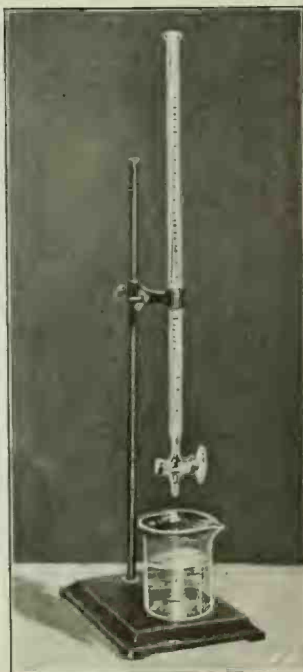
Fig. 128. Method and Apparatus of Quantitative Determination of Chlorides in Water. A Standard Silver Nitrat Solution is Added to the Water.
