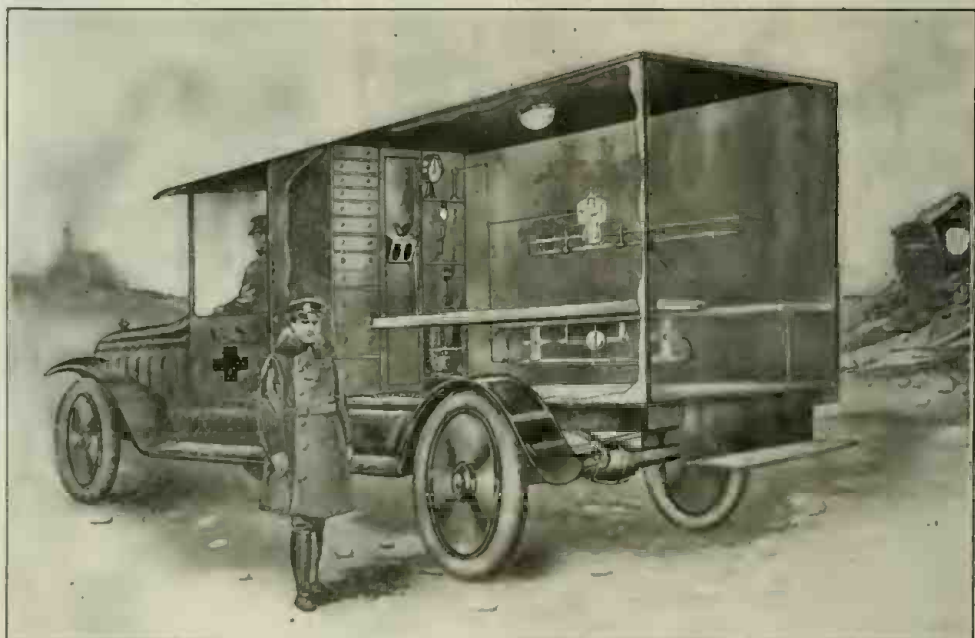
The Latest Design of Portable X-Ray Ambulance for U. S. Army. It Derives Its Power, About Two Kilowatts, from a Special Dynamo Driven by the Engine. It Includes Plate Developing Facilities, Complete Switch-Board for Controlling X-Ray Bulbs, and Other Necessary Conveniences.
